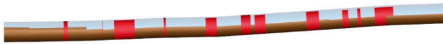
Figure 13: Slug flow formation diagram in the pipeline under a certain operating condition.
